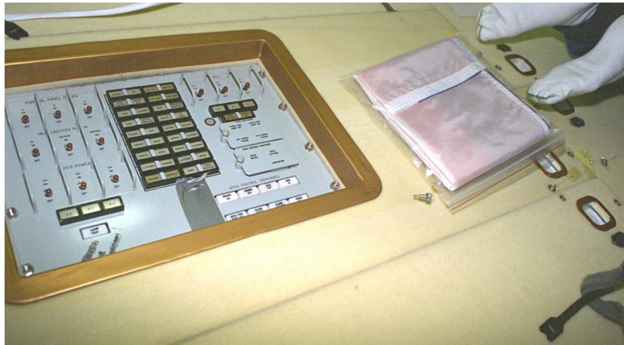
Figure MOD-95 Docking Module's APDS Panel
