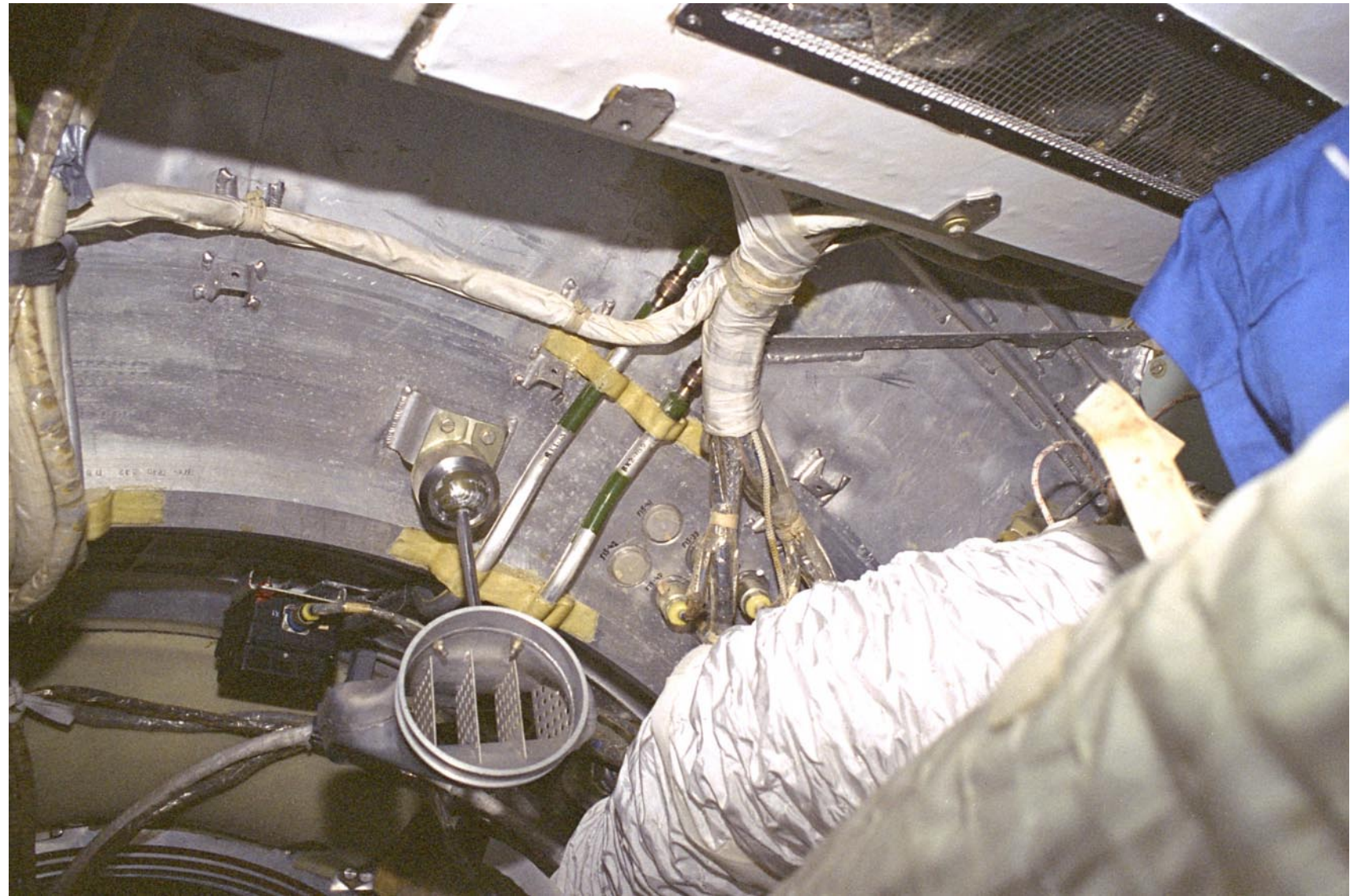
Figure MOD-35 Directional Air Vent in the Transfer Node End of Priroda
