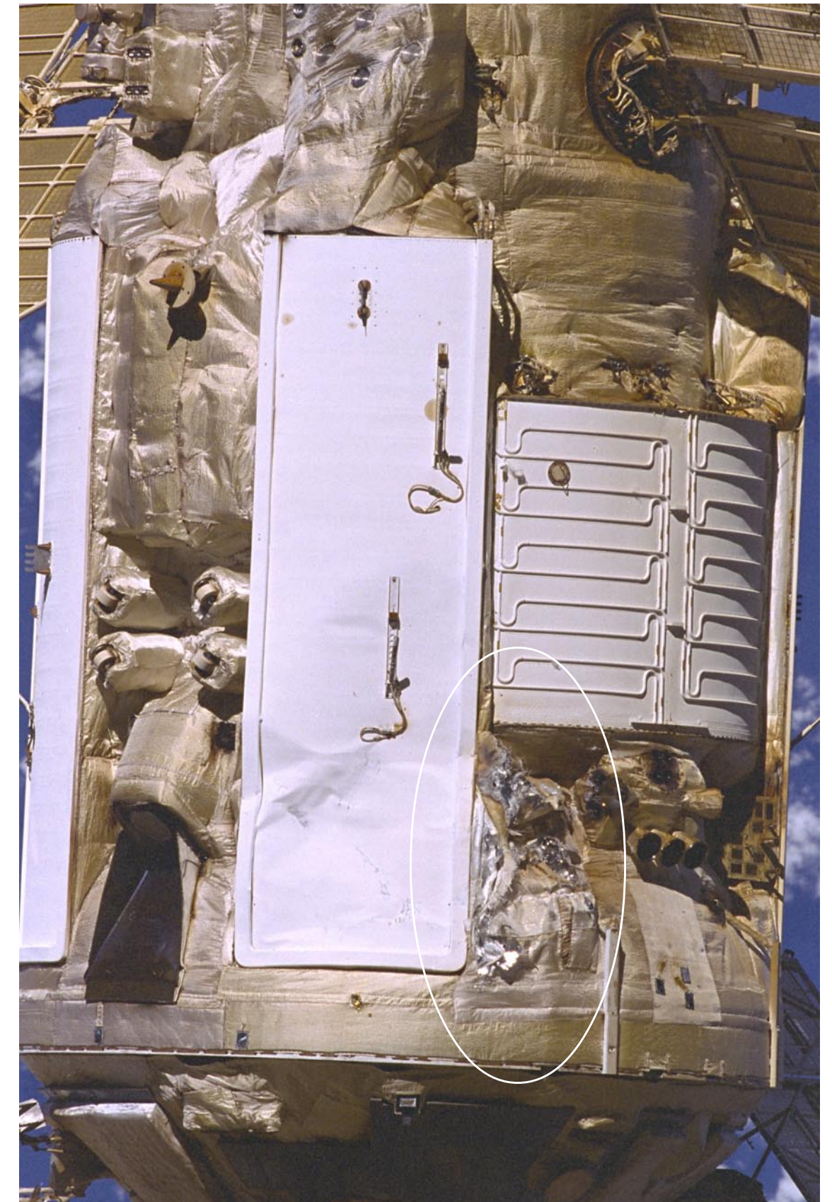
Figure MOD-59 Damaged Radiator on Spektr and MLI Cut to Find the Leak
