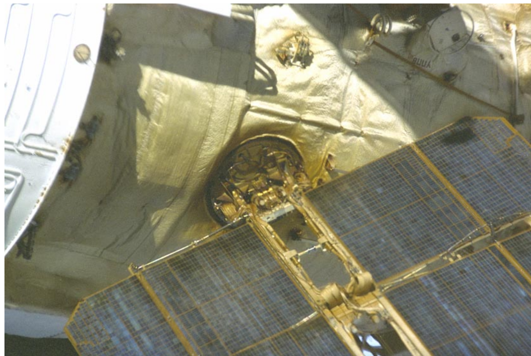
Figure MOD-57 Spektr's Solar Array Drive
